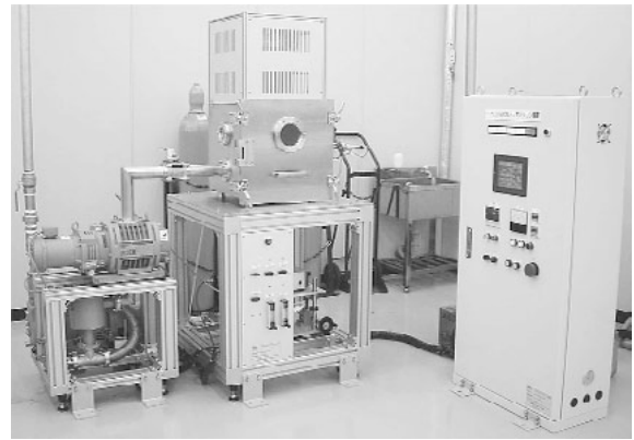
Fig. 9 Photograph of an Aerosol Gas Deposition system.
