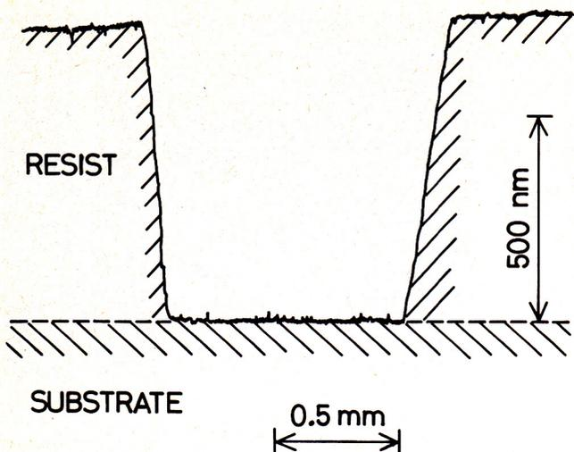
Fig. 5. Micro-depth profile scanned across a ditch.
