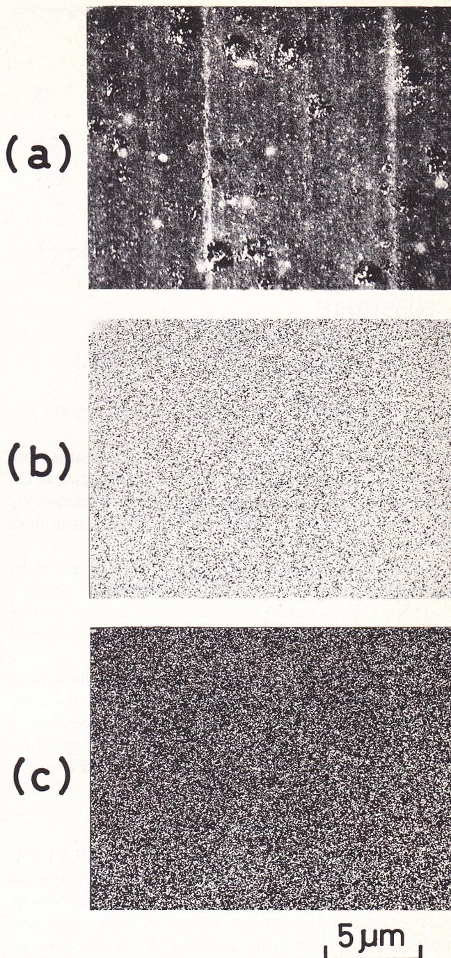
Fig. 4. Specific X-ray emission image for the mixed deposit of Fe-Ag UFP; secondary electron image (a), FeK<sub>α</sub> X-ray image (b) and AgL<sub>α</sub> X-ray image (c). Spot size is φ3 μm. (20 KV, 0.03 μA)
