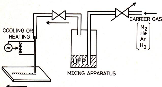
Fig. 1. Arrangement of the spray deposition for surface conditioned UFP (partial oxidation).
