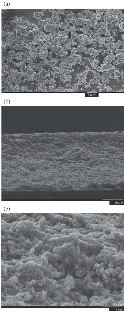
Fig. 2. (a) SEM micrograph of the BR-QZ (7.4 μm) powder. (b) SEM image of cross section of deposited film obtained from BR-QZ (7.4 μm) powder. (c) High-magnification image.
