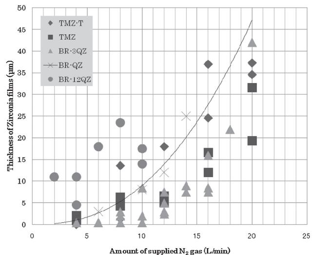
Fig. 4. Summary of the relationship between the film thickness and amount of supplied gas.
