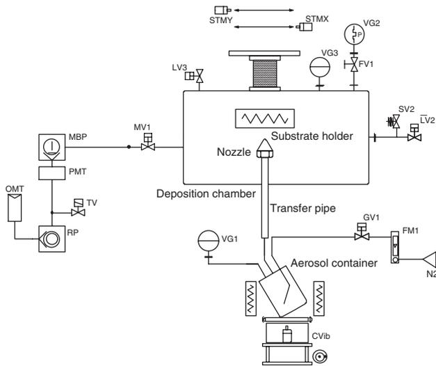
Fig. 1. Schematic diagram of the AGD apparatus.
